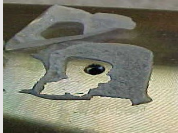
Epoxy Adhesion Failure
