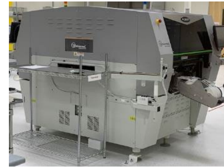
Universal Instruments Pick and place (+ wafer feeder for die attach)
