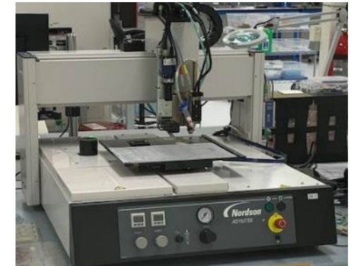
Nordson Asymtek (dep and epoxy encapsulation for LEDs)
