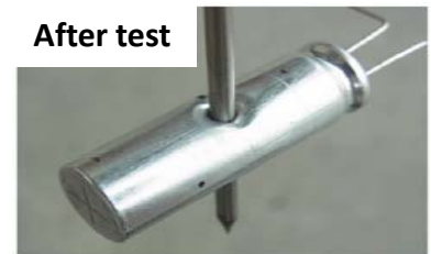
Nail penetration test
