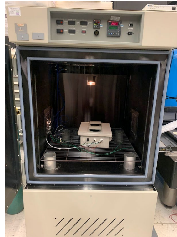
Profiling station placed inside environmental chamber
