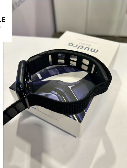
Mudra band brain computer interfacing using a combination of bipotential sensing, including 'surface nerve conductance' IDTechEx photo.
